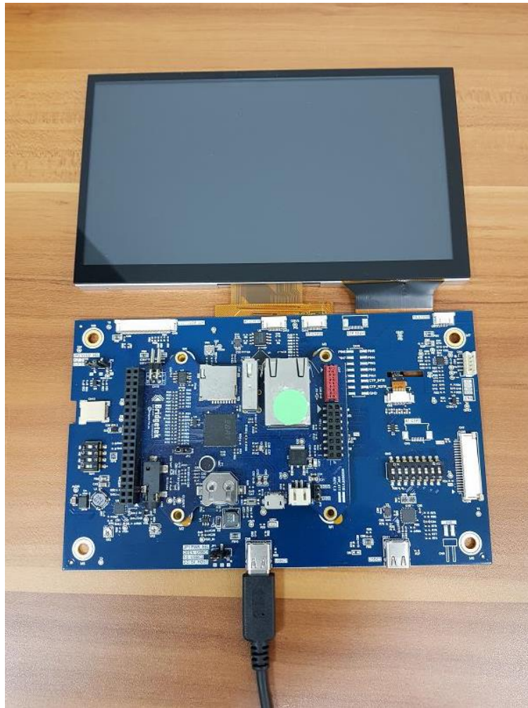
Figure 5-1 – MM900 setup with 7" 1024x600 panel
