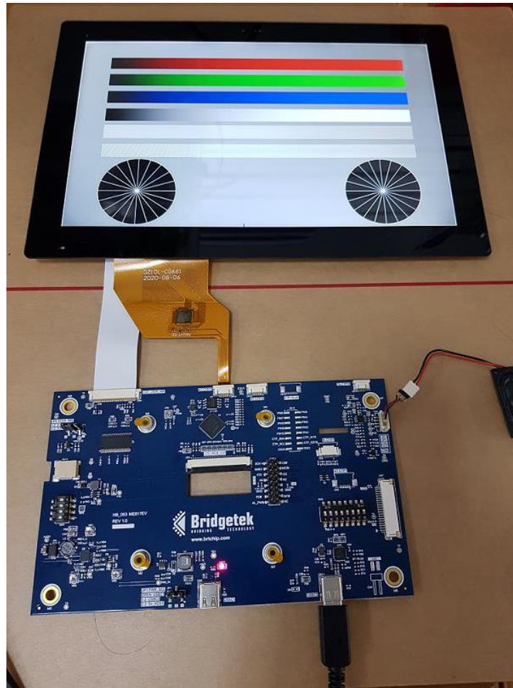
Figure 5-4 - PC setup with 10.1" 1280x800 panel
